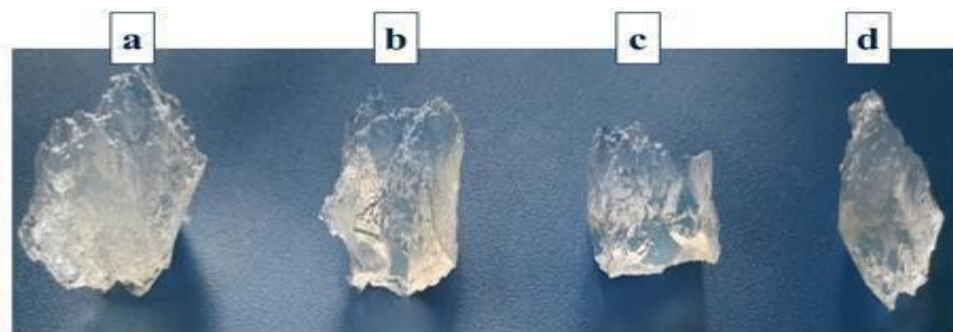
Figure 2: Swollen PVA/CMC hydrogels prepared via the two-step (a and b) and the in-situ (c and d) methods
